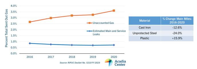
Rhode Island Unaccounted for Gas vs. GHG Inventory Estimated Gas Main and Service Leaks + Gas Main Replacements by Material Type
